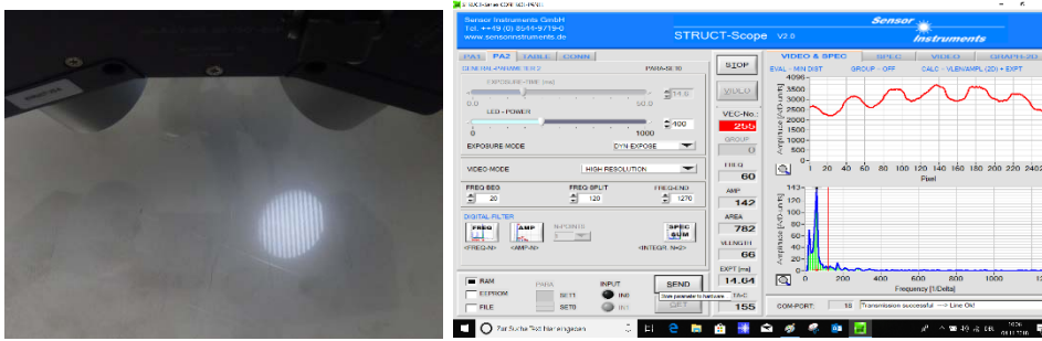
The gloss sensor GLAST-85-30°/30°-DIF-1.0/1.0 - all three settings with the PC surface STRUCT-Scope
